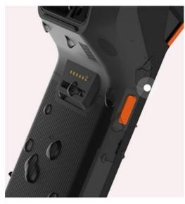
Rubber seals added to the edges of the paper bin, charging port, and earphone port help prevent water, oil and dirt damages. Even in a restaurant with a lot of oily smoke and water stains, it can protect the device for continuous and stable operations.
