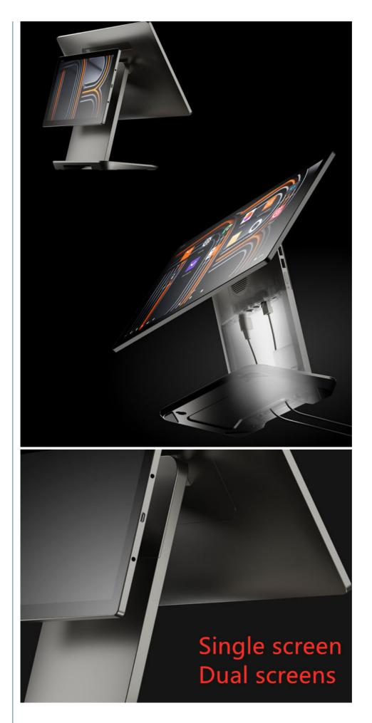
Elevate customer interactions with a stunning 15.6" FHD (1920×1080) display boasting 400nits brightness and anti-fingerprint coating. Ideal for high-traffic environments, the screen resists smudges while delivering vibrant visuals. Pair it with the optional capacitive touch monitors for interactive kiosks or digital menus. With 8MP front-camera capabilities and 2W stereo speakers, engage users with crisp video calls and
